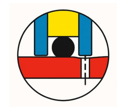
Figure 6 Undercut bore and polish
