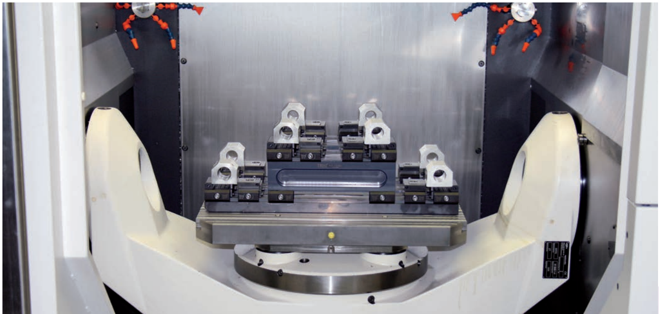
Eight parts being machined on three faces in one operation.
