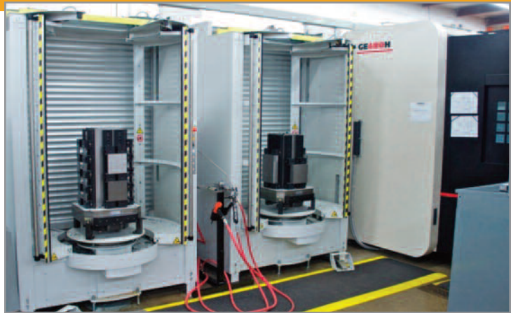
AME workholding tombstone devices on an Enshu HMC at TRD. 56 block sizes are run, producing over 450 different parts, in one-off to 500-piece quantities. The HMC runs in tandem with a Fastems 10-station (5 x 2) pallet changer.
