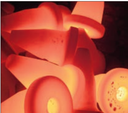
Typical parts forged at Clifford-Jacobs weigh 3-800 lbs. and include gears, axles, valve bodies, hubs, rings and clevises. Short runs and production contracts to 15,000 pieces annually are executed.
