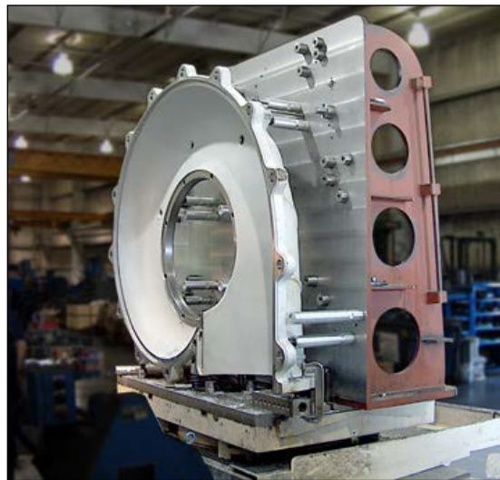
Slurry pump housing mounted to a dedicated fixture
