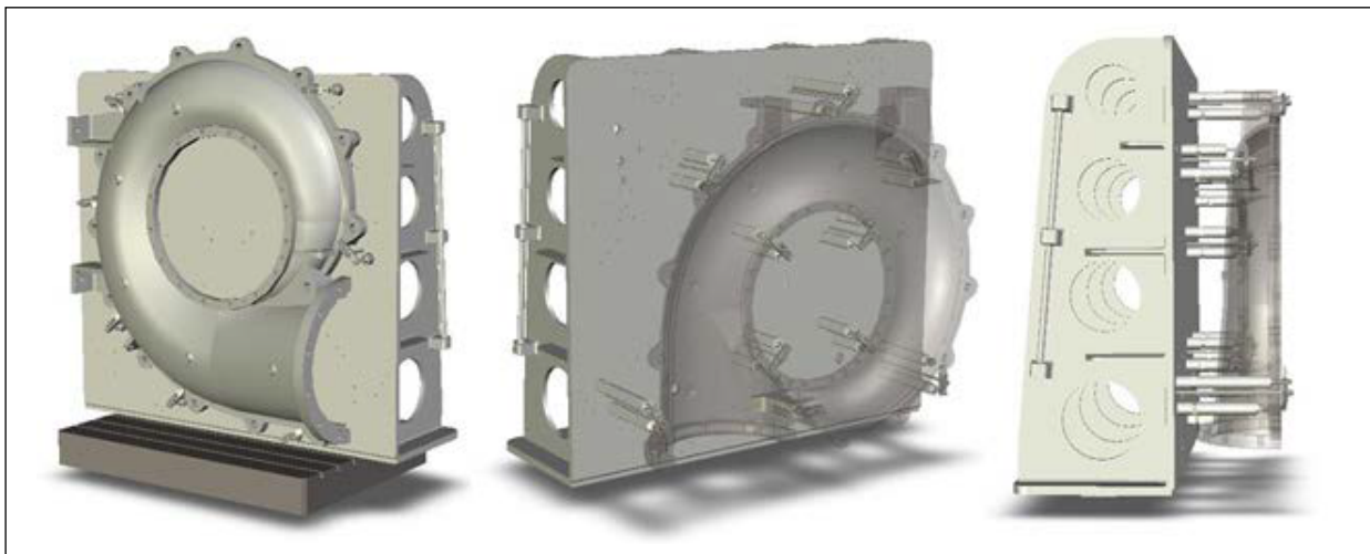
Image 1: CAD models of the two halves of the slurry pump housing on the fixture.
