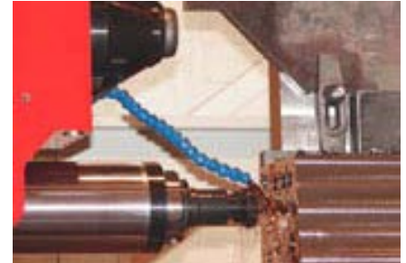
As the machine uses BTA/STS or inserted gundrill tooling for the highest penetration, the OTT-Jakob drawbar, drilling spindle and toolholder maintain accuracy at full extension.
