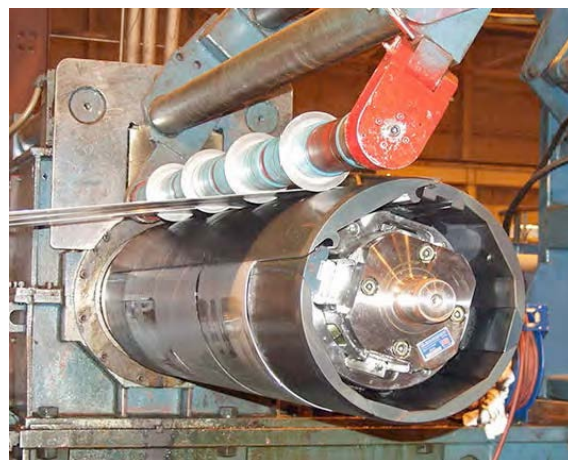
Aeromet mandrel shown with steel material rolled onto it; the drawbar taper is visible on the exposed end.
