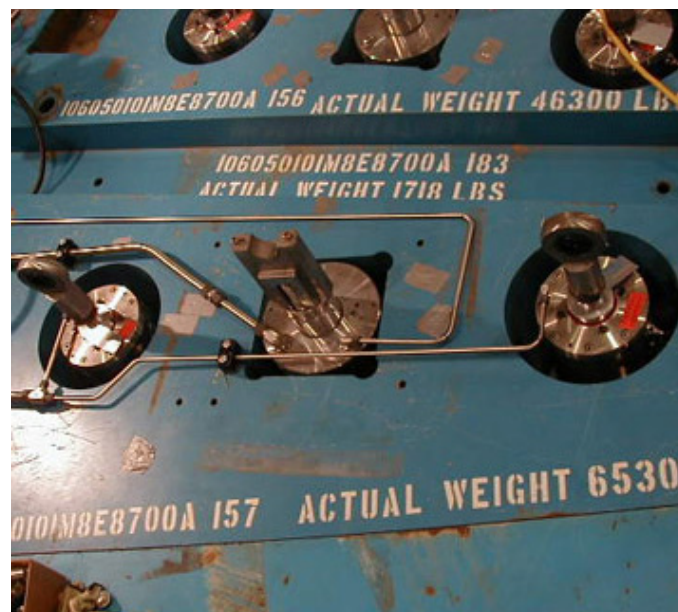
View of shutter top with bridge beam removed, showing the lift cylinder (center) and Sitema Safety Catchers (left and right)
