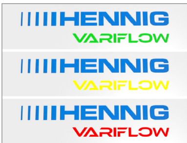
STATUS LIGHT • On (green) • Idle (yellow) • Warning (red)
