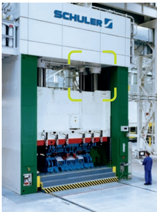
Hydraulic press Safety Catcher as DGVV-approved restraint device
