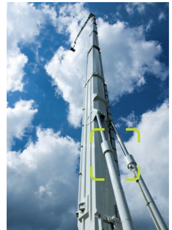
Mobile elevated work platform Securing the telescopic arm of the 101 meter high work platform
