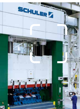
Hydraulic press Safety Catcher as DGUV-approved restraint device
